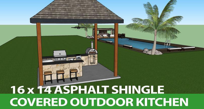
This outdoor living space features a 16 x 14 foot outdoor structure, 4 foot concrete pad, asphalt shingle covered roof, an outdoor ceiling fan, granite countertops, and stone veneer. Blaze Outdoor Products for this kitchen include a 40 inch built-in propane grill, grill cover, 39 inch door and triple drawer combo, 4.1 cu. foot compact refrigerator, refrigerator trim kit, built-in propane power burner with lid, and a roll out trash drawer.
