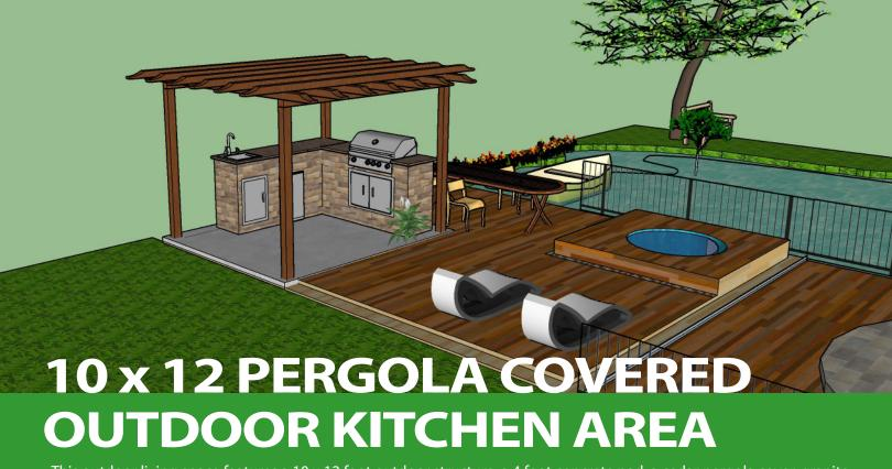
This outdoor living space features a 10 x 12 foot outdoor structure, a 4 foot concrete pad, a cedar pergola cover, granite countertops, and stone veneer. Blaze Outdoor Products for this kitchen include a 40 inch stainless steel built-in propane grill, grill cover, and a 40 inch access door with a paper towel holder.
